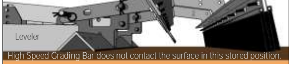
High Speed Grading Bar does not contact the surface in this stored position.
