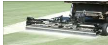
The rear rubber mat can be used when incorporating top dressing. Or, it's quickly removed with two quick pins.
