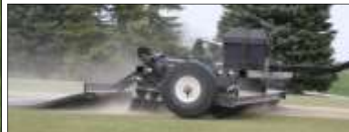
The rear rubber mat can be used when incorporating top dressing. Or, it's quickly removed with two quick pins.
